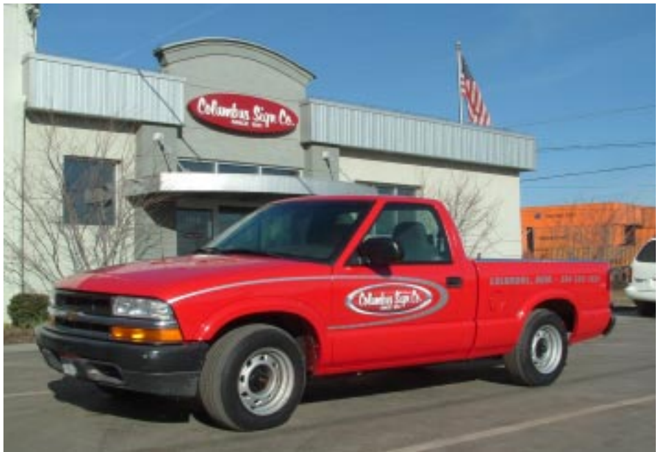
Columbus Sign's truck and building logo imprints were produced on its EDGE FX, using Gerber 3M Scotchcal 220 protective laminated film. The building sign is painted aluminum with Gerber Sabre routed push-through illuminated letters.
