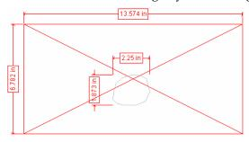
The larger dimensions represent the overall size of the image in Composer. The smaller dimensions are the clipping path.
