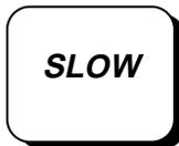
Use the SLOW key to access slow slew mode. Slow slew mode moves the platen or tool one step at a time, which simplifies precise registration of artwork produced by the GERBER EDGE™. In normal or slow mode, the platen or tool move continuously as long as the arrow keys are pressed.
