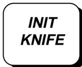
Use the INIT KNIFE key to initialize the swivel knife so that the blade faces 0°. Press the INIT KNIFE key after loading the swivel knife and selecting swivel knife mode.
