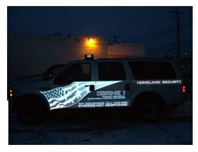
Using a flag design printed on Gerber 280i Reflective with the Gerber EDGE. Troy wrapped the SUV with graphics that clearly identify it both day and night. (see photos)
